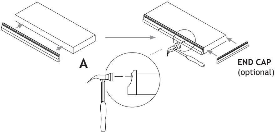
\* If END CAP will be installed replace the trim with the one supplied in the END CAP set F23C
