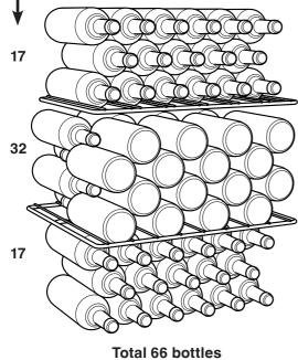
$\underline{/!}$  Important The maximum load per grid shelf is 45 kg.
